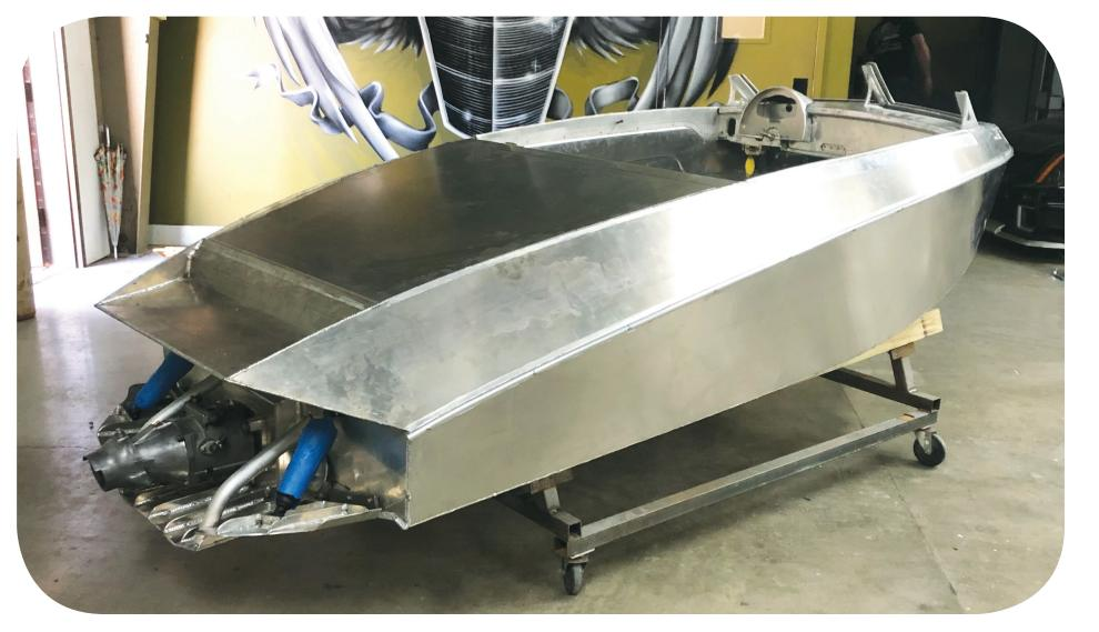
Our hulls are cut out of .1875" and .125" marine grade aluminum 5052 making them the perfect balance between strength and light weight.
